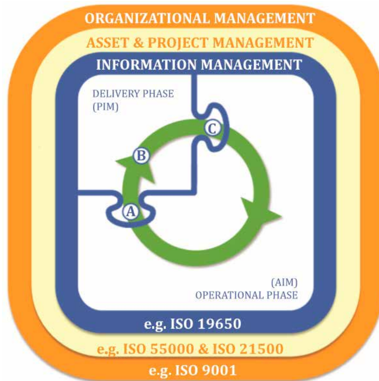
Figure 1: Information management lifecycle as it relates to ISO standards, according to ISO 19650
