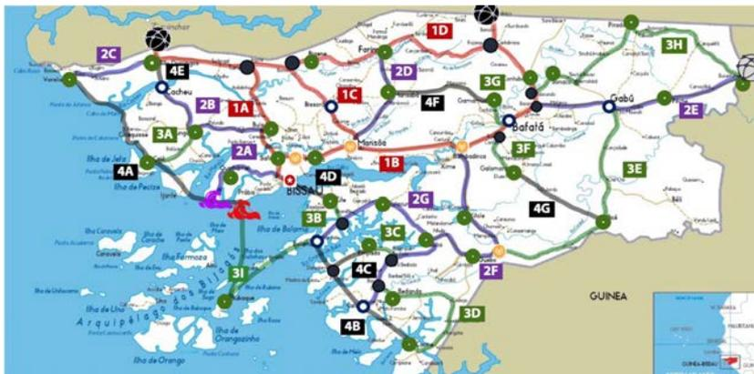
The proposed network layout of **2.877 km** of fibre cable, covering over 99% of the population, is based on technical assumptions, traffic forecasts, and existing and planned infrastructure. It consists of **four implementation phases** and connects **56 designated nodes**.
